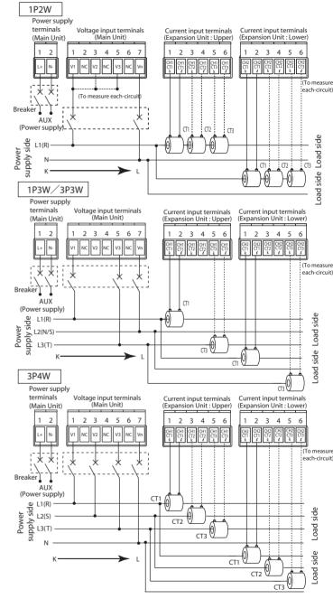
⚠ Vn terminal should be connected to N-phase which is grounded.
